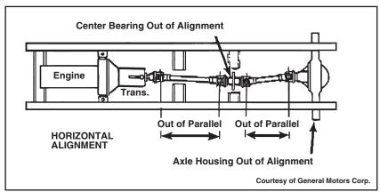
**Horizontal Alignment of Drive Shaft**
