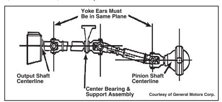
Phase Alignment of 2-Piece Drive Shaft (3-Piece Shaft is Similar)
