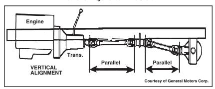
**Vertical Alignment of Drive Shaft**
