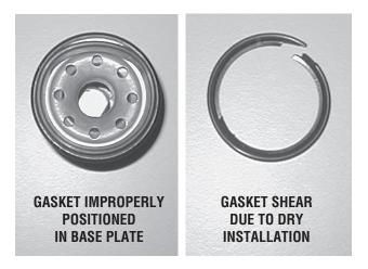
The above illustrations reflect a gasket improperly positioned in the base plate retainer and gasket shear due to a dry installation. Major oil leakage is certain with either condition.
