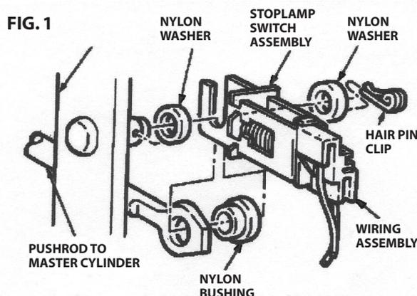
Someone had improperly installed the assembly, which incorporates bushings, washers and a stop
