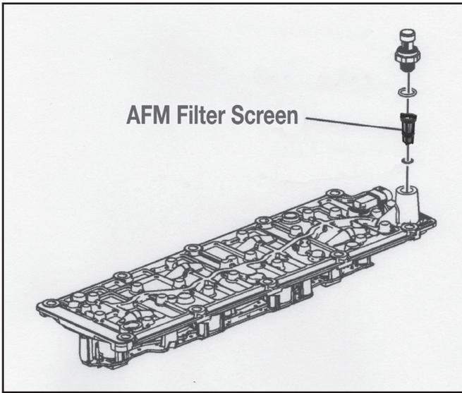
FIG 2: Valve Lifter Oil Manifold
