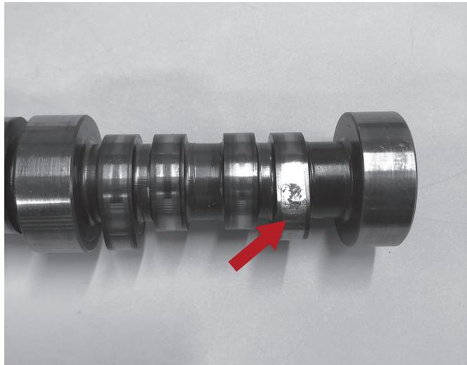
FIG 3: Camshaft Lobe Wear
