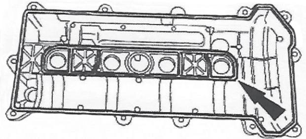
**Fig. 1 - Internal Valve Cover Gasket**
